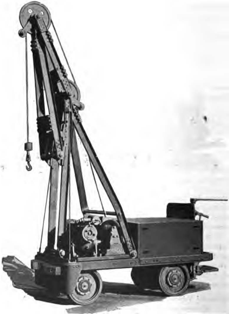
FIG. 6.—4,000-LB. STACKING CRANE WITH 13-FOOT LIFT
